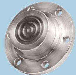
D-12 PULP SEAL,FLOATING RING TYPE Min Pressure :-30inHg Max.Pressure:600 psi
